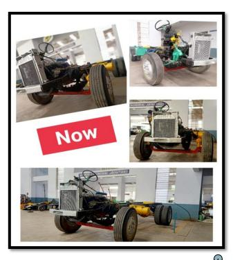
*New Feather added in Automobile laboratory*: An old non working rusty dumper truck was turned into a valuable & useful component to demonstrate the "Heavy Vehicle Chassis and Driveline Systems" to the students.
