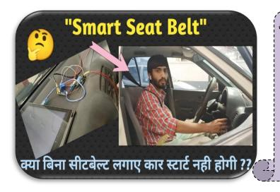
Ansh Shah: Final year student has developed "Smart Seat Belt" system to ensure safety to the driver by wearing of seat belt. Systems of this project work in such a way that, car's engine won't start unless driver wears a seat belt. Project was funded by SSIP. Guiarat.
